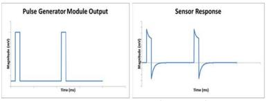
4. Reconnect the sensor output to the alarm circuit after the self-test has terminated. Any residual current from the applied pulse will be discharged.
