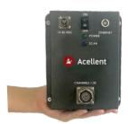
The DARTTS Hardware is a compact and lightweight passiveactive hardware that powers the sensor system and feeds data back to the SHM-DARTTS software in real-time. In combination with the software and SMART Layer sensors, this system integrates impact detection with active damage scanning and trajectory estimation.
