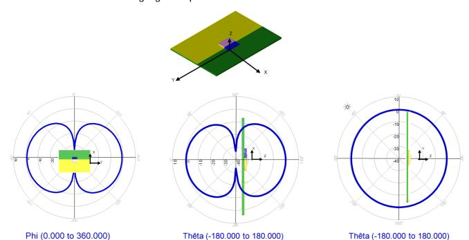
Gain measurement in dBi @ 2.45 GHz.
