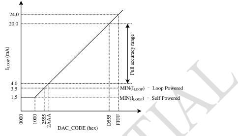
Figure 4.7 Loop current transfer function
