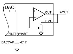
Figure 4.4 Configuration for voltage output mode
