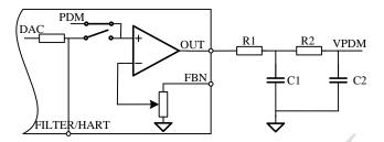
Figure 4.9 RC filter for PDM output
