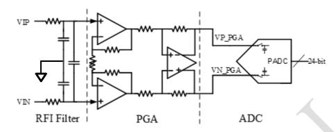
Figure 4.2 Primary signal channel (PGA+ADC)
