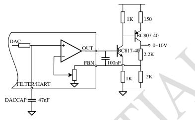
Figure 4.5 Configuration for 0~10V output mode
