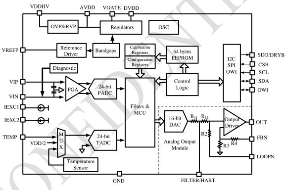
Figure 4.1 Block diagram of the NSA2860
