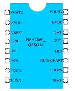
Figure 6.1 SSOP-16 package pin configuration
