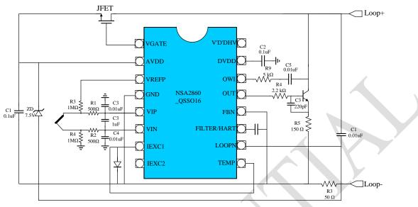
Figure 7.6 Thermocouple  $4 \sim 20$ mA temperature transmitter
