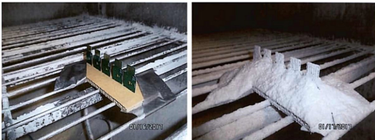
Figure 13 Vesper piezoelectric MEMS microphones mounted on test boards, before (left) and after (right) an IP5X dust test
