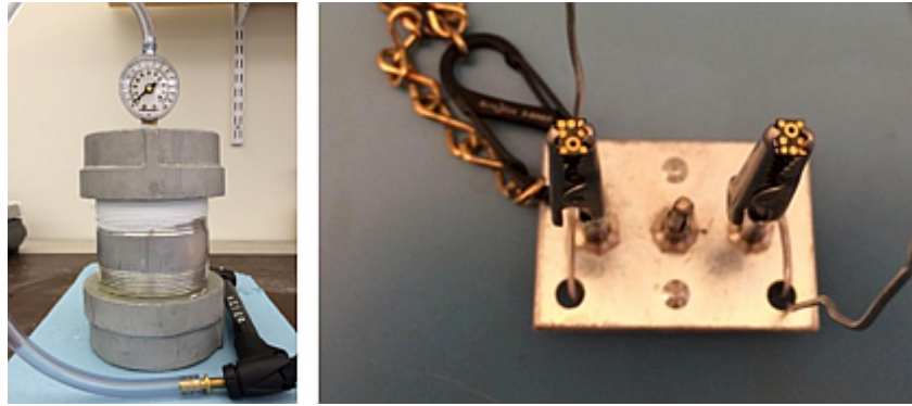
Figure 15 Microphone water-testing apparatus (left), microphones tested with acoustic ports face-up (right)
