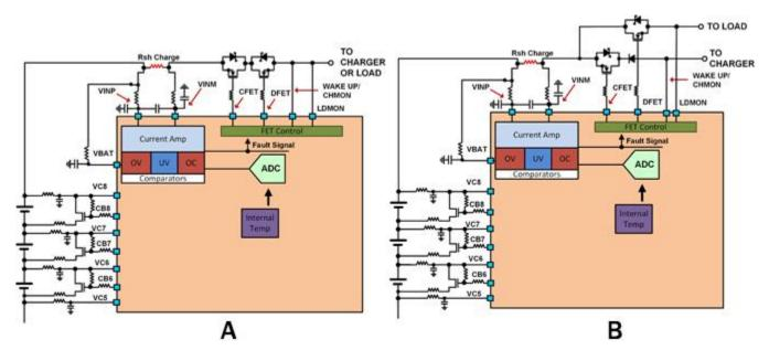
Figure 2. Cutoff FET Schematic Illustrations for (A) Single Connection for the Load and Charger; (B) Two Terminal Connection that Allows for Charging and Discharging Simultaneously
