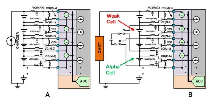
Figure 3. Different Types of Cell Balancing (A) Bypass Cell Balancing FETs are Used to Slow the Charge Rate of a Cell During the Charge Cycle; (B) Active Balancing is Used During the Discharge Cycle to Steal Charge from a Strong Cell and Give the Charge to a Weak Cell
