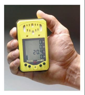
instruments offer quick, push-button calibration with electronic corrections in place of older potentiometer adjustments.
